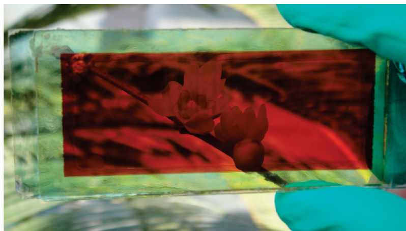
Figure 6. Digital photograph of a large-area bifacially active transparent DSSC fabricated in this work. The cell was sealed with Surlyn, and the electrolyte was introduced through a drilled hole on the counter electrode.
